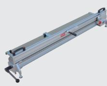
Max. sheet metal thickness: Galvanized steel Aluminum, Copper, Zinc 1.00 mm (0.039 in) Stainless steel
